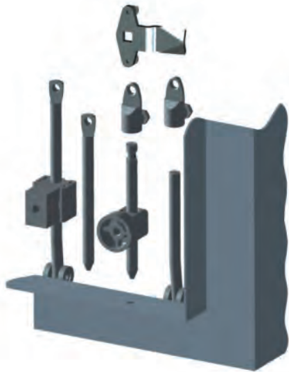
Drive mechanism: Cam
